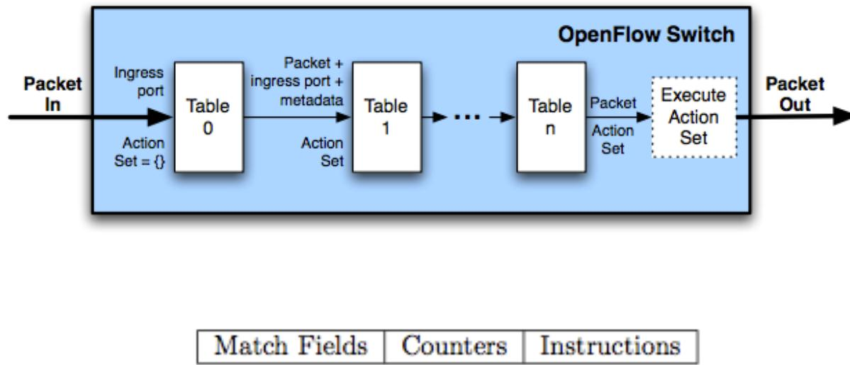
Table 1: Main components of a flow entry in a flow table.
